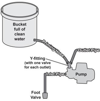
1. Connect a bucket full of at least 3 gallons of water to one side of the Y-fitting using a hose, as shown above. (If available, a continuous water supply, such as a spigot, may be used instead.) The bucket must be positioned higher than the pump's outlet.
